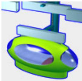
worst extremes of weather and can travel at speeds up to 30-40 miles per hour. The load capacity depends upon the type of vehicle. A standard people JPod can carry four people with a generous margin on normal weight.
