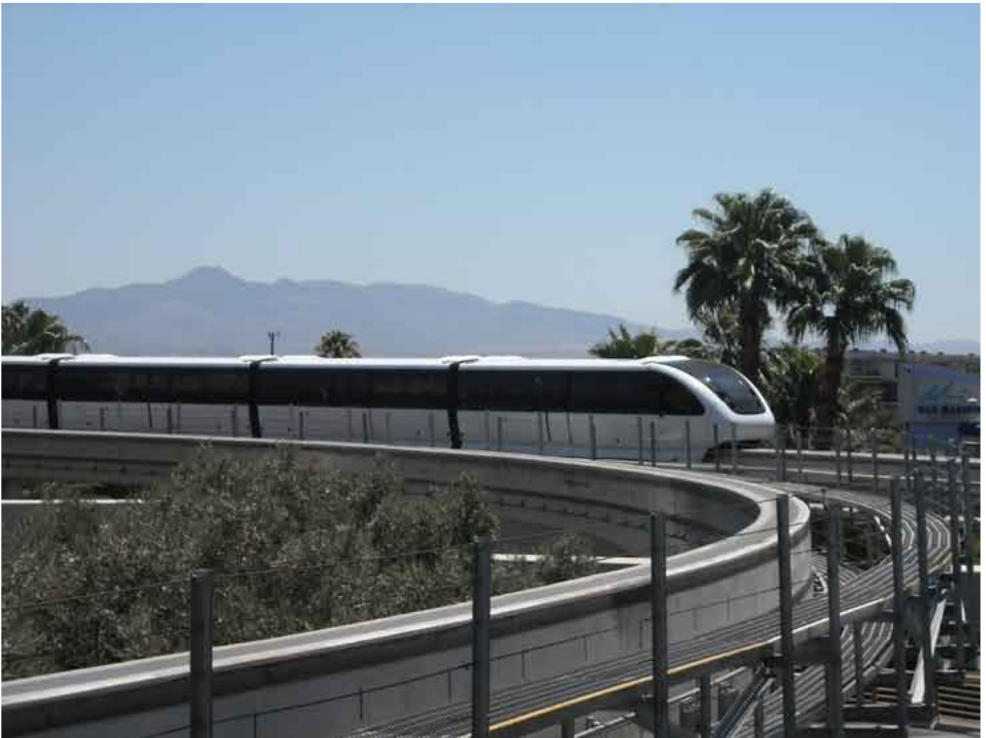
The Monorail's four, completely automated, Bombardier trainsets allow frequencies as low as two minutes, at more than 99 percent reliability.
