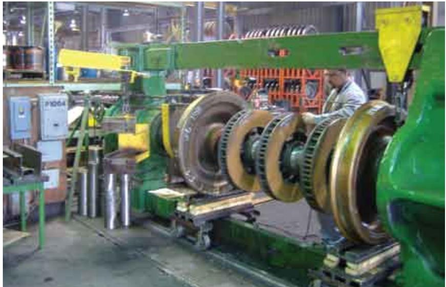
Scott Dively (above) assembles a wheel set for an Amtrak Acela coach car. Acela wheel sets are unique in North America due to their three brake discs.
