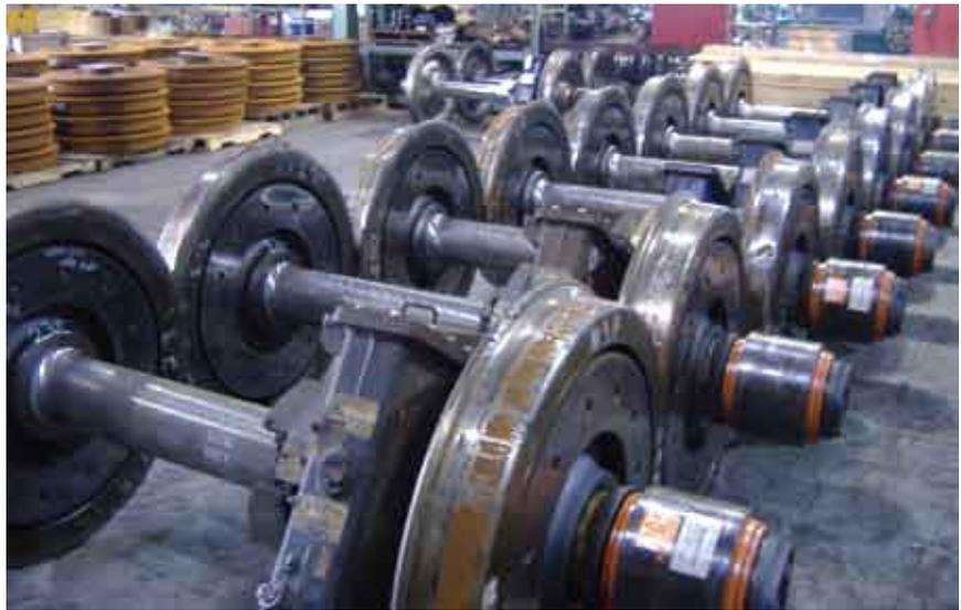
Long Island Railroad M-7 railcar wheel sets with disc brakes are mounted to the wheels (above). Below, the first wheel set assembled for PATH’s new PA-5 vehicles is distinguished as the First Article Inspection (FAI), which will be the indisputable template for all other wheel sets assembled under the contract. It will also be the last wheel set delivered to PATH.
