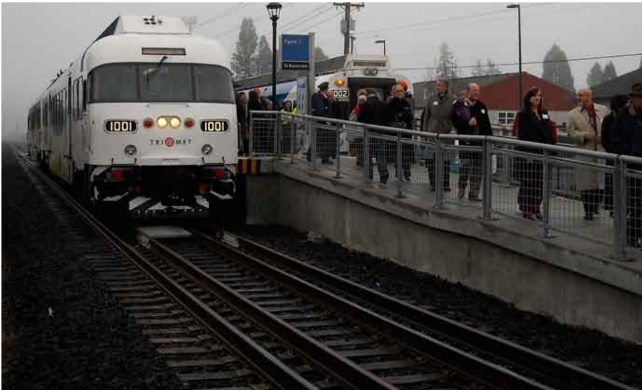
Station bypass tracks – like those installed at the Tigard Station shown here – allow appropriate clearance for the Portland & Western's freight trains to pass the high-level platforms used at WES stations.
